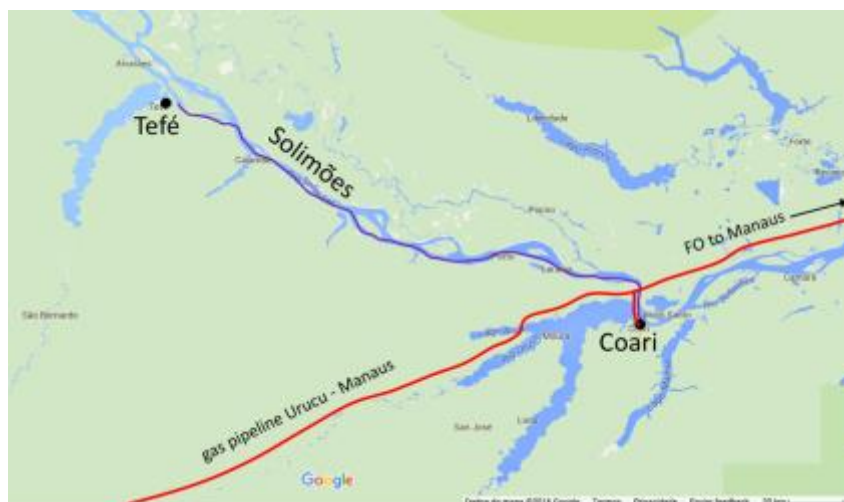
Figure 17: The pilot project linking Coari to Tefé along the Solimões.
