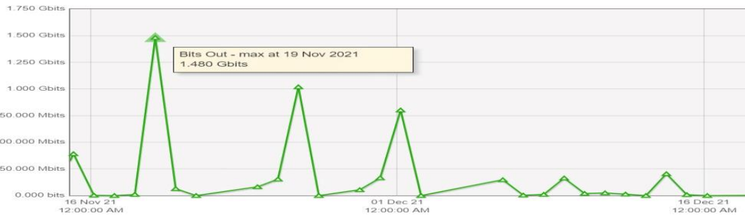
Figure 10 – Statistics of AUTH's live streaming network throughput (one streaming engine)
